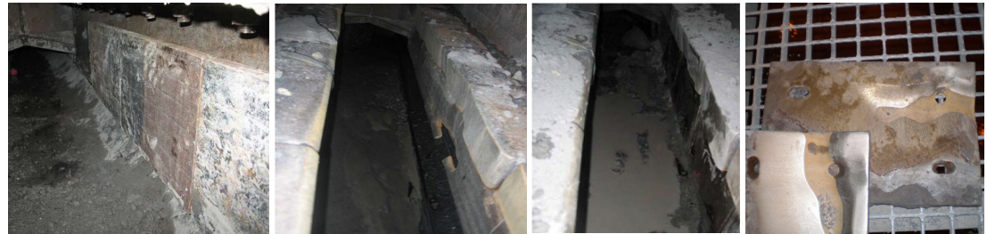
Overlay liner wear plates at installation
