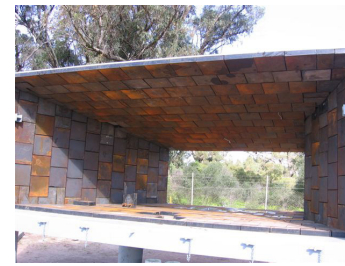
Laminite® Rubbadex liner wear plates at installation
