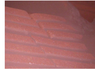
Same Laminate® wear plates 8 months & 2 million tonnes later
