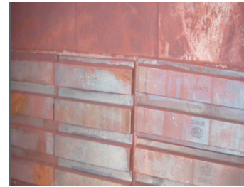
Laminate® Rockbox liner wear plates at installation
