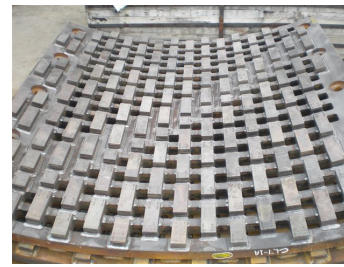
New Breaker Screen
